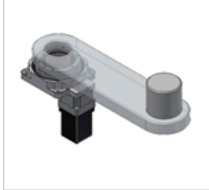
Applications where a moment load is applied
